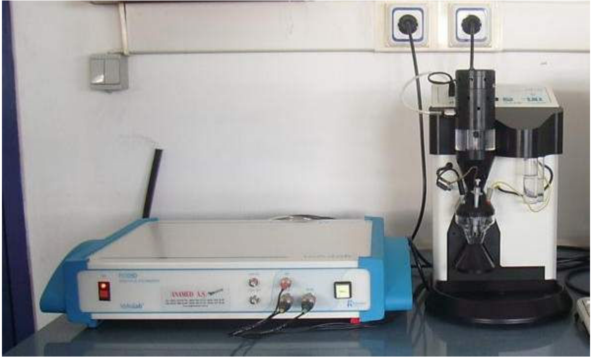
Şekil 3.1 Radiometer marka Voltalab 50 (PST050) Analitik Potansiyostat ve Radiometer marka MDE150 Polarografik Stand
