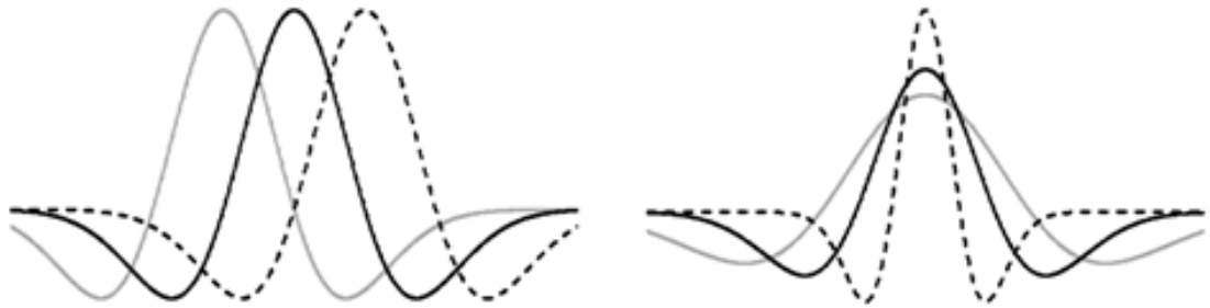
Figure 9 : Translation and dillation of a wavelet (Source: Rua, 2011)
