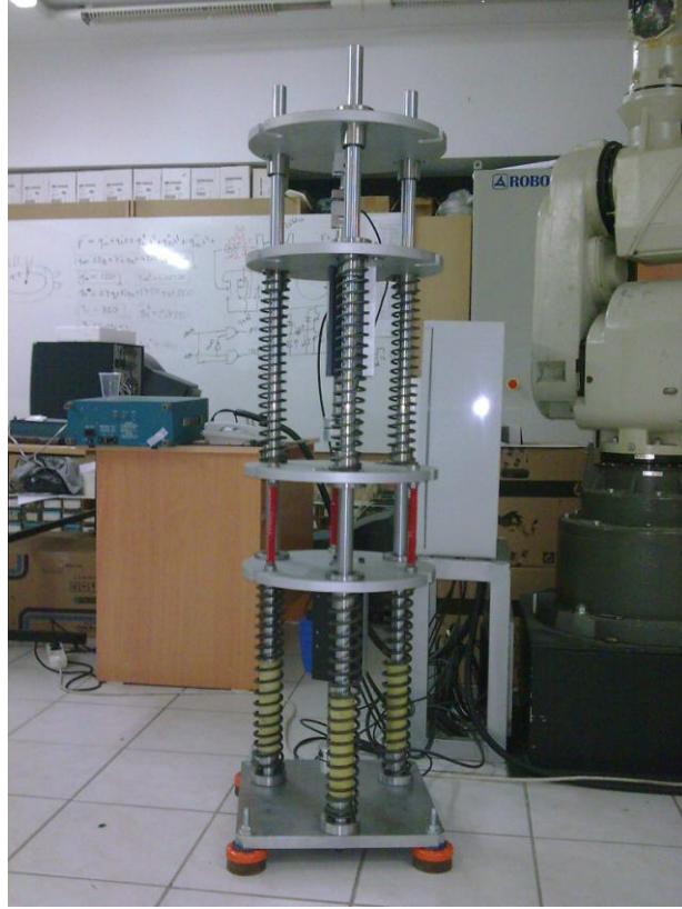
Figure 5. 5 Active suspension system experimental model.
