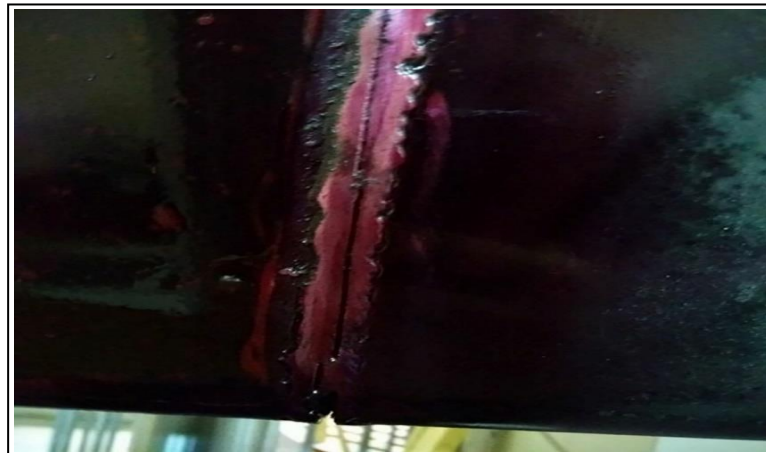
Figure 3.13 Extended fatigue crack thickness along butt-welded connections
