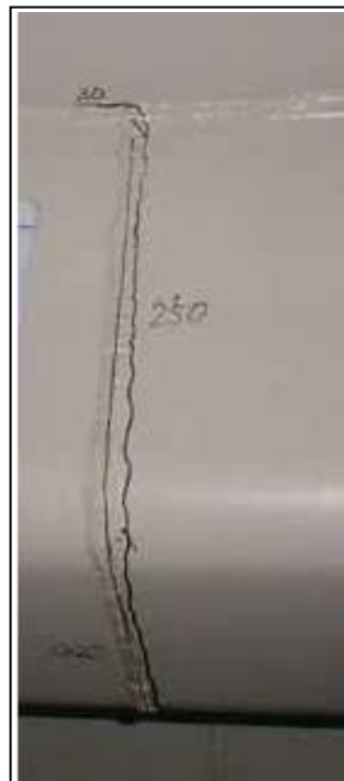
Figure 2.8 Visual identification of a rib splice weld root crack [75]
