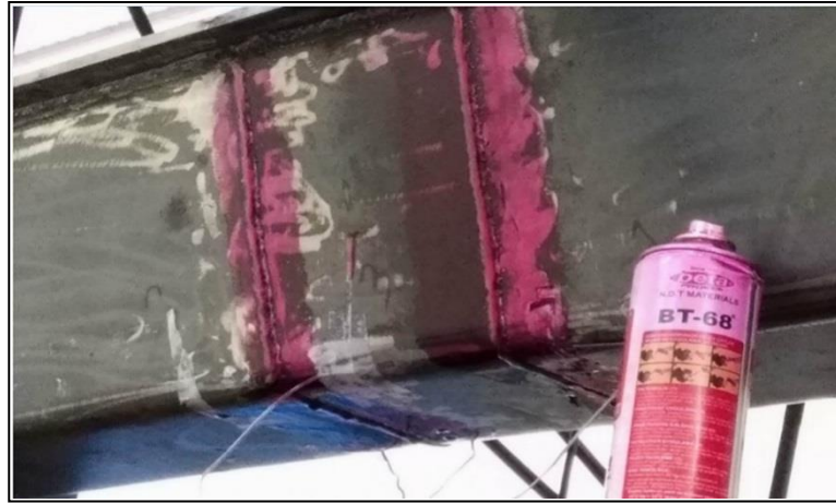
Figure 3.12 Detection of crack propagation using a dye-penetrant method
