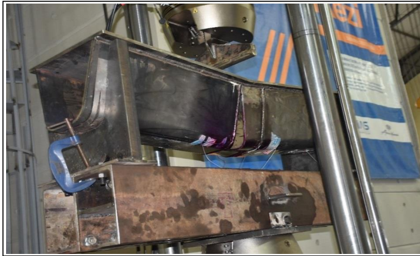
Figure 3.10 Failure mode at the bottom of the rib
