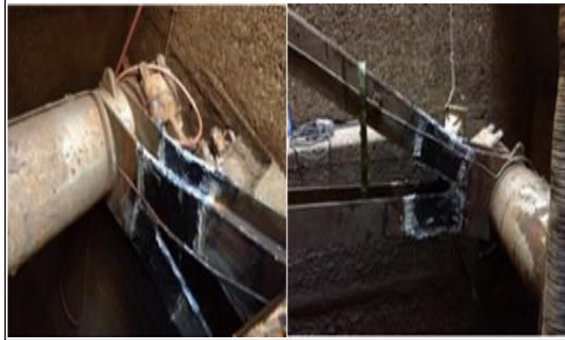
Figure 2.11 Cracks in valve's strut arms (flange and flange-web) [93]
