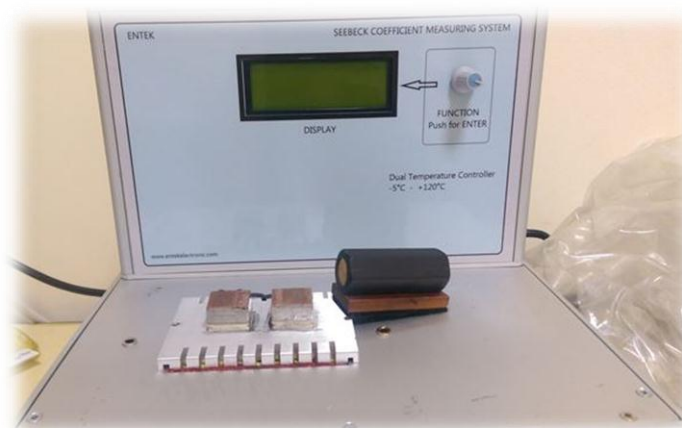
Figure 3.2 Seebeck coefficient measuring system.
