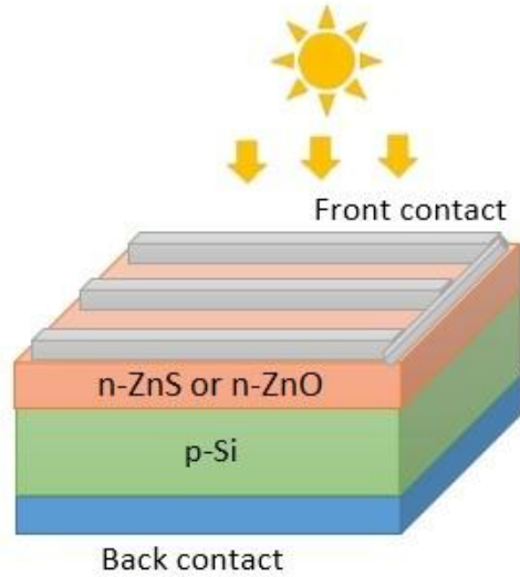
Figure 4.5 Schematic diagram of n-ZnS/p-Si or n-ZnO/p-Si heterojunctions
