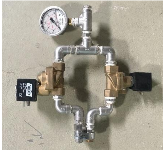
Figure 3.5 Two Nozzle System with the LNN and GG-W Nozzles
