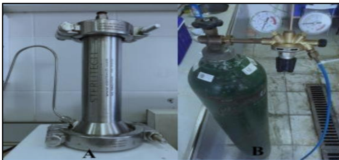
Figure 3.6 The dead-end mechanism (A), the nitrogen tube used in the experiment (B)
