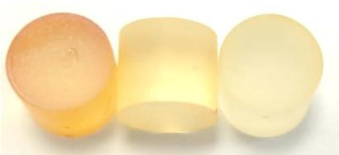
**Figure 2.5** Pure epoxy specimens used in experiments
