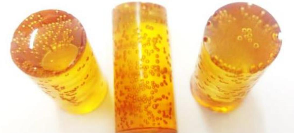
**Figure 2.3** Pure epoxy specimens obtained with the first method
