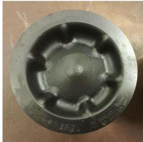
**Figure 2.20** Volvo wave piston model [16]
