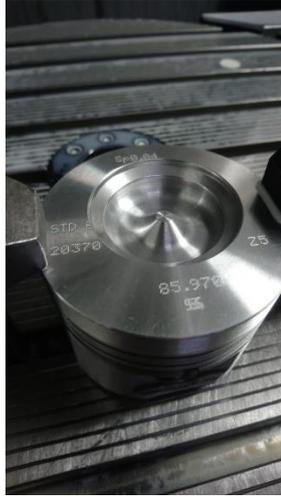
**Figure 4.3** Machined stepped lip combustion chamber
