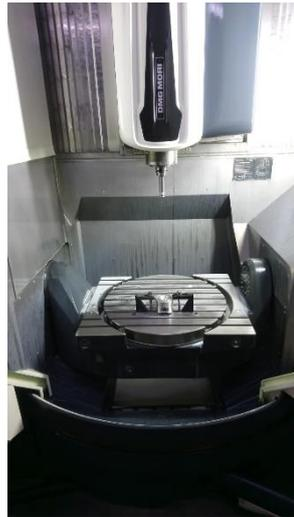
**Figure 4.2** Machining process of stepped lip bowl
