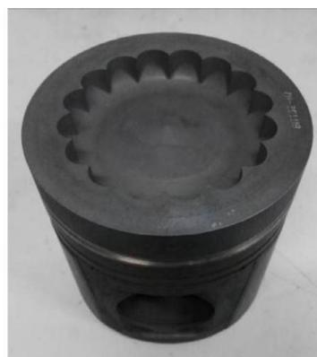
**Figure 2.21** Lateral swirl combustion chamber [17]
