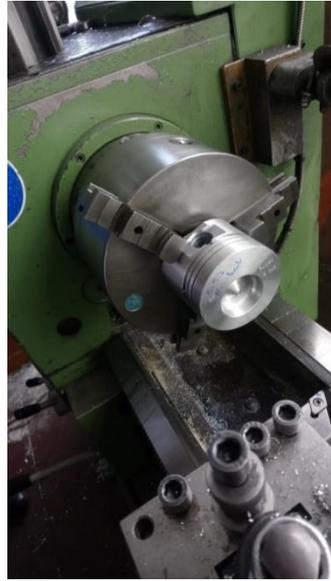
**Figure 4.5** Top surface machining process of the second piston
