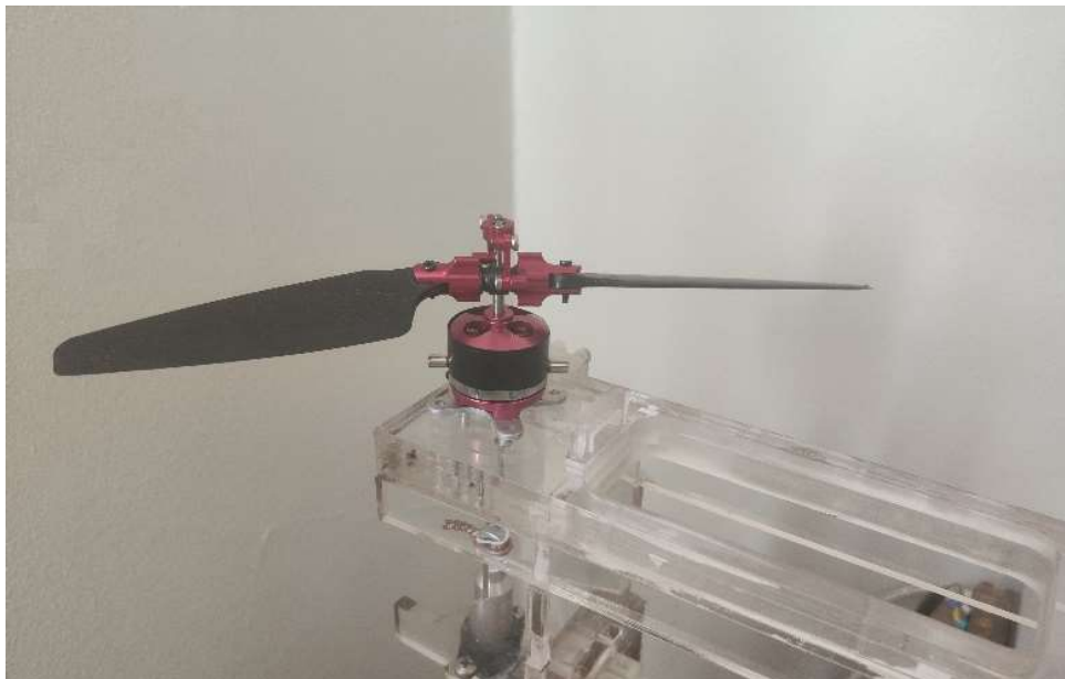
Figure 3. 8 The Variable-Pitch Mechanism and Corresponding Propellers
