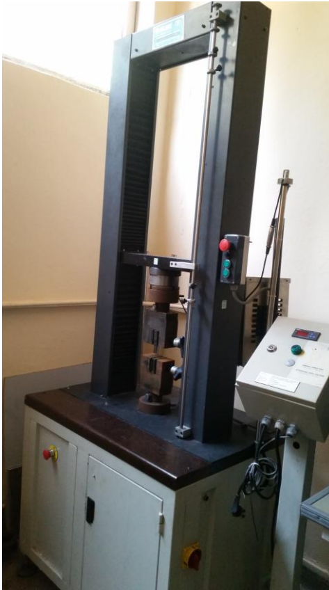
Figure 5.17 Electro-mechanical Testing Device used for Tensile Tests
