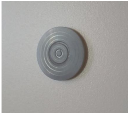
Figure 5.20 Disc type wear test specimen of base material
