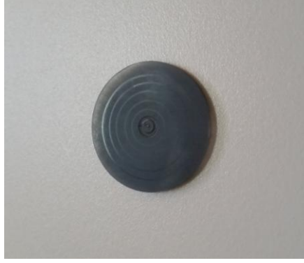
Figure 5.21 Disc type wear test specimen of CNT reinforced composite material
