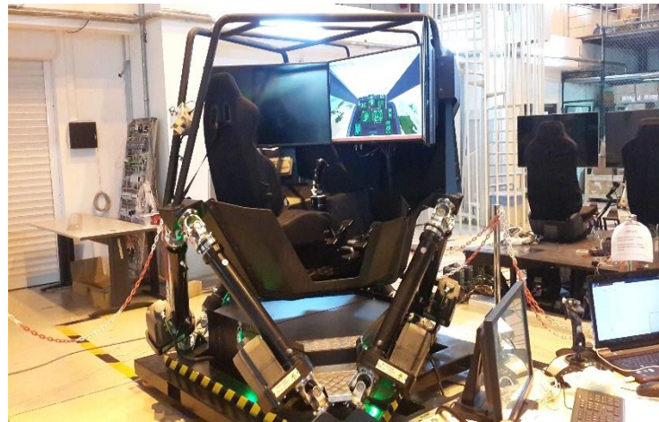
Figure 2.2 6 DOF Stewart Platform Structure
