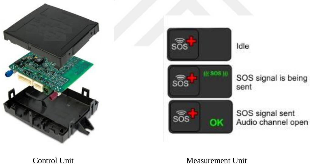
Figure 4.2 eCall Component Hardware [161]
