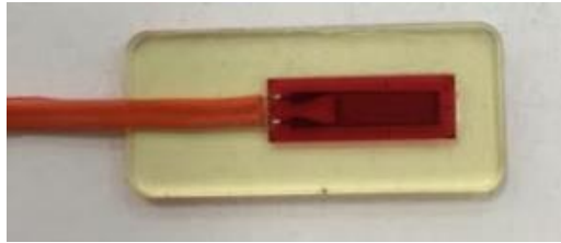
Figure 3.6 Sample of strain gauges
