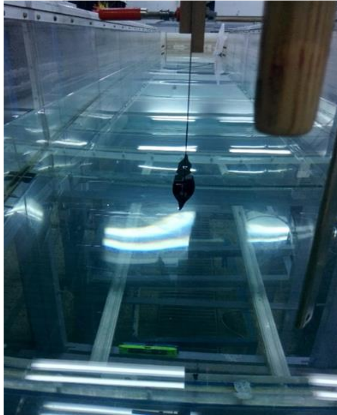
Figure 5.1 Close-circuit water channel and printed squid model
