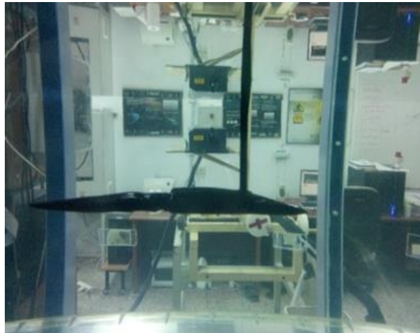
Figure 5.3 1,600 \times 1,200 pixels spatial resolution CCD camera seeing the printed squid model from the bottom
