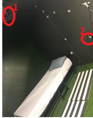
Figure 2.5 The setup of the experimental environment with two different radar locations
