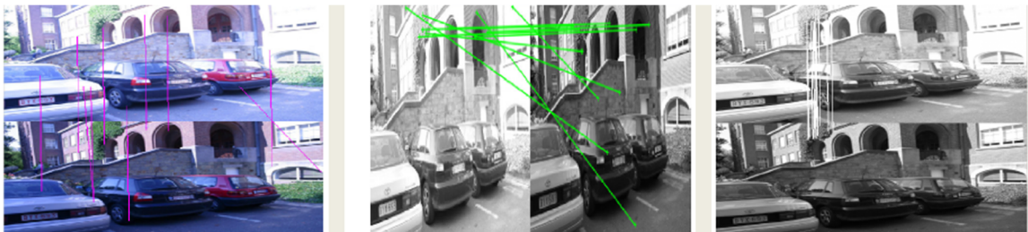
Figure 2.4 Images matching in different illuminations [29] Left: using SIFT. Middle: using PCA-SIFT. Right: using SURF
