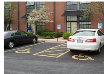
Figure 3.34 Accessible Parking with Wheel-Stop (Type A Spaces) [66].
