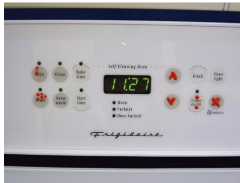
Figure 3.13 Microwave oven controls using indicator lights with added fluorescent Braille markings, San Diego Center for the Blind [28].
