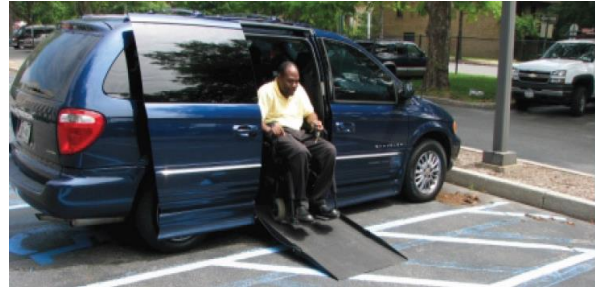
Figure 3.33 Accessible Parking Spaces which have a type (A & B) Spaces, and Access Aisles [67]; and Van Parking Side Exit Ramp (Type B Spaces) [66].
