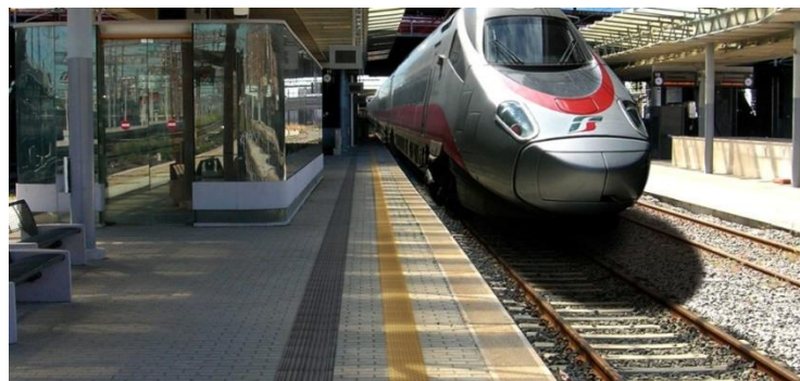
Figure 3.12 Tactile paving for the visually impaired which means a line of orientation, guidance, and safety [55].
