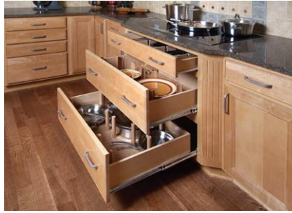
Figure 3.11 Design application, drawer storage adjusts for a variety of pan and dish sizes, from ASID Atlanta Show Home [28]
