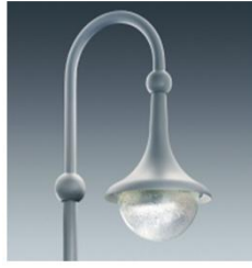
5LA15622KG101 decorative outdoor luminaire housing made of glass fibre reinforced polyester painting in black (RAL 9005) clear glass Degree of protection: IP 54 Protection class: II Mounting type: pylon annex
