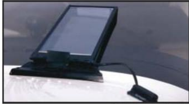
Electrically heated windshield
